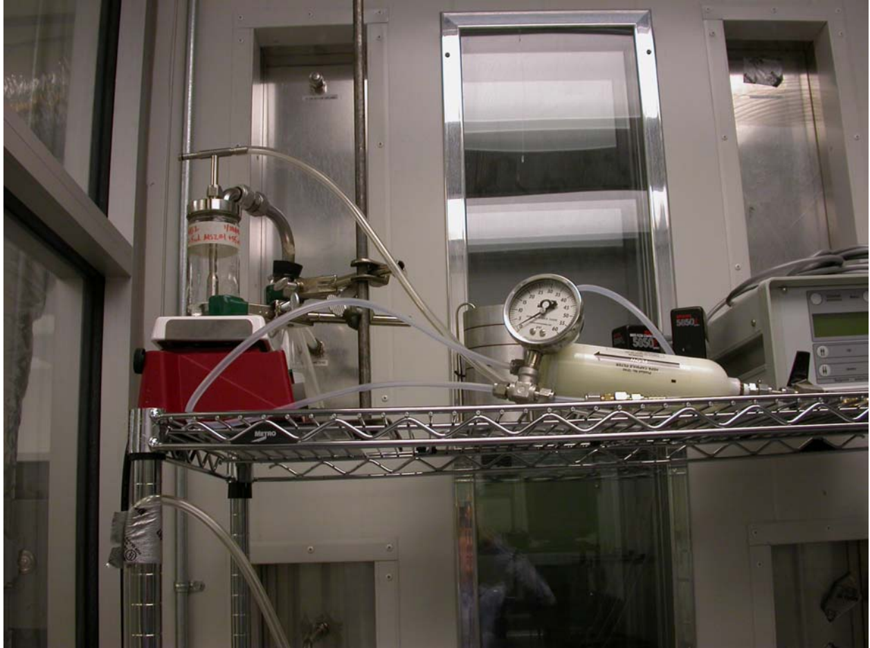
Photograph 1. View of Bioaerosol Generation Components. The glass collision jar, fitted with a nebulizer, is visible atop a magnetic stir plate. HEPA-filtered air (HEPA capsule visible near center) is supplied through tubing to the nebulizer at regulated pressure to aerosolize the microbes. The output of the collision nebulizer is directed through the glass drying flask and into the injection port in the chamber wall.
